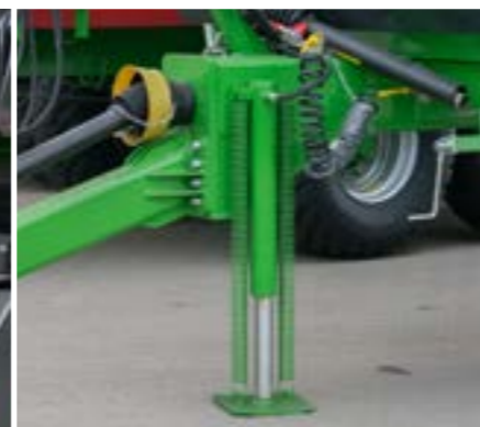
Simple and very practical - hydraulic support leg
