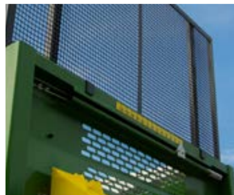
Height indicator of the rear wall
