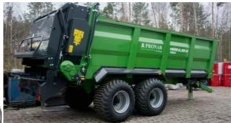
Strong and robust – the body of the N262/1 model has a height of 4'2" | 1265 mm and capacity of 494 ft 3 | 14 m 3 .
